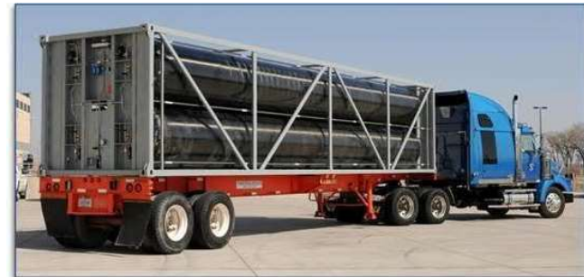
Tube Trailer From " www.energy.gov/eere/fuelcells/hydrogen-tube-trailers "
